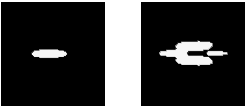
Figure 22 One and two source image reconstruction using holographic method
