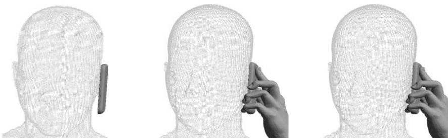
Figure 1. Woman (Ella) head model with phone, a) without hand, b) with hand position 1, c) with hand position 2.
