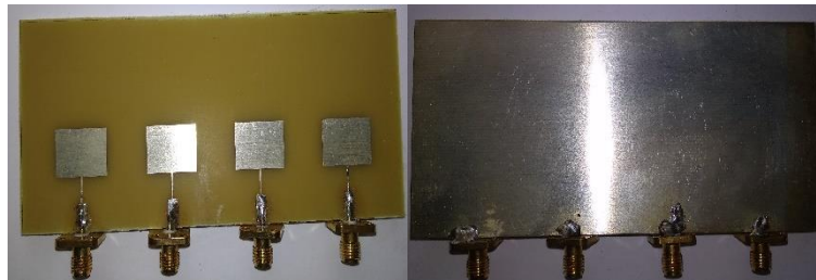
Figure 8. Photograph of fabricated setup of PMAA for mutual coupling measurement. (a) Front view (b) Back view.
